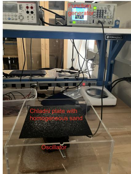
Figure 1: Experimental Setup
